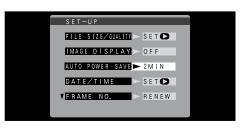
Once you enable this function, the monitor is temporarily switched off to reduce power consumption (Sleep mode) if the camera is not used for about 30 seconds. If the camera is then left unused for a further time (2 or 5 minutes), it is automatically switched off. Use this function when you want to get the maximum possible running time from the battery.
